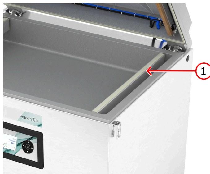
Figure 16: Replacing the Silicone Rubber of the Silicone Holders
